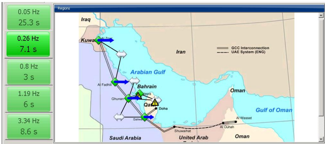
Figure 17 - Mode Shape of 0.26Hz mode in Observed Part of the Network
